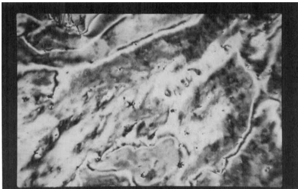
PHOTOMICROGRAPH I. Compound 18 in the smectic C phase at 202°C. See Color Plate II.
